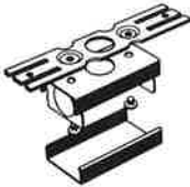
TK 116 Top entry wiring box for TKN or LTN continuous runs TK 1181 Similar to above for LTR
