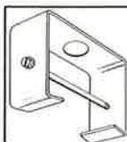
FCM 4509 Auxiliary Suspension Bracket
